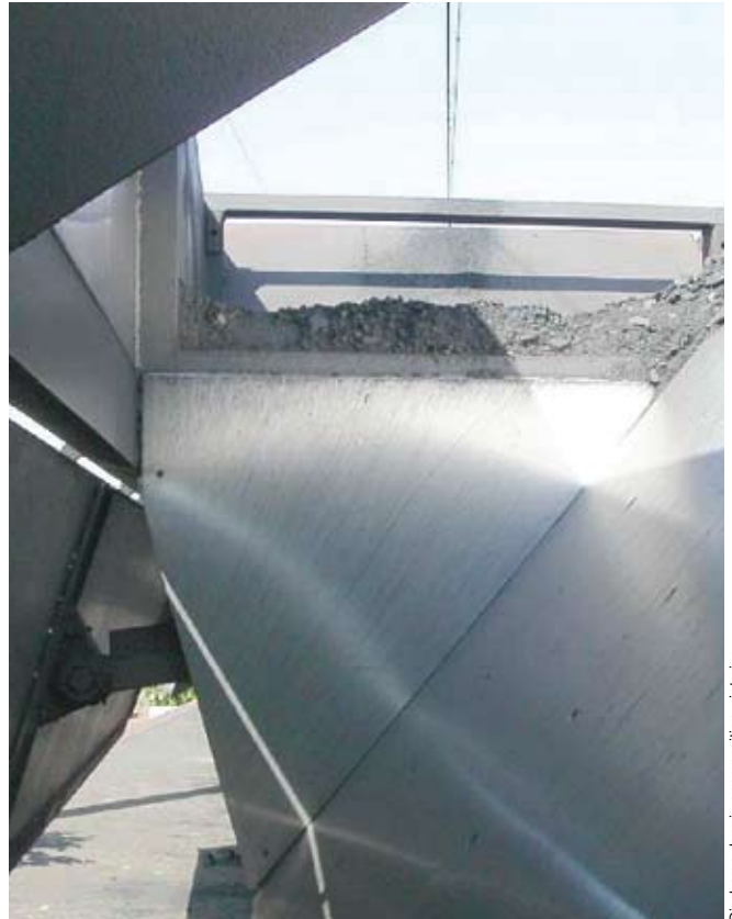
Discharge door in open position – interior.
