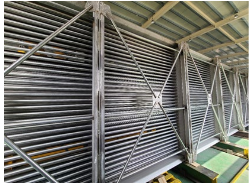
Fig. 3 GGH bundle made by 329J4L LBW tube Courtesy of POSCO
