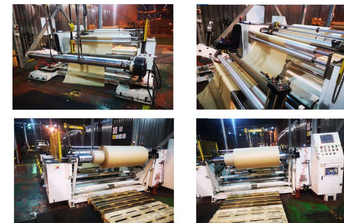
Figure 2: Zhongtai Line - ZTM-B1600 Slitter rewinder (2018)
