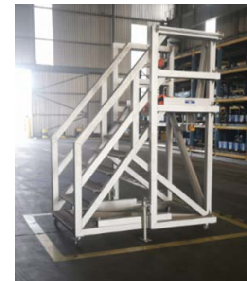
The ladder is stored in demarcated area when not in use. Brakes are engaged and the downriggers are retracted.
