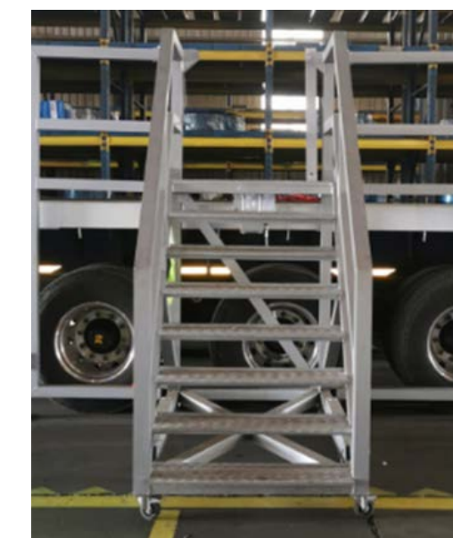
Examples of the ladder once attached to a trailer before the person can climb on, for stability.
