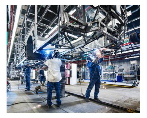
Overton insisted that 3CR12 was used despite this not being their standard material of choice. It proved to be a wise decision as Adams and Overton recall that a 3CR12 MAN bus which was manufactured in 2000 was stripped in 2010 with no rust to be found anywhere. This durability is also evident in the 16-18 year old buses that the Company was recently able to sell.
