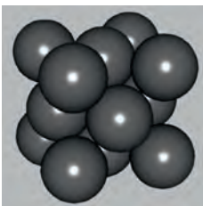
Atoms in a face-centered austenitic structure
