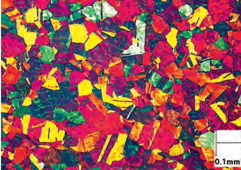
Micrographic view of the austenitic crystal structure of chromium-nickel stainless steels
