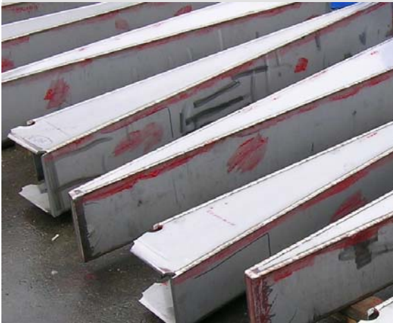
Figure 7: Pickling paste applied to weld areas to remove contaminants and oxides
