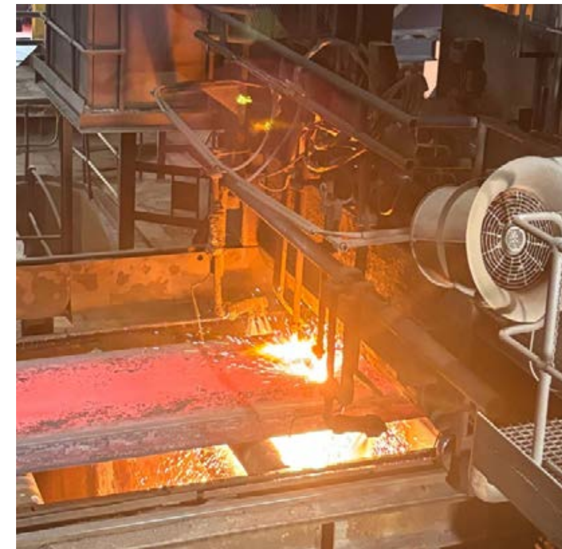
Normal slab cutting
