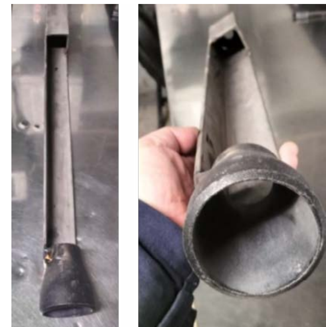
Fig. 4. Tool manufactured according to the design
