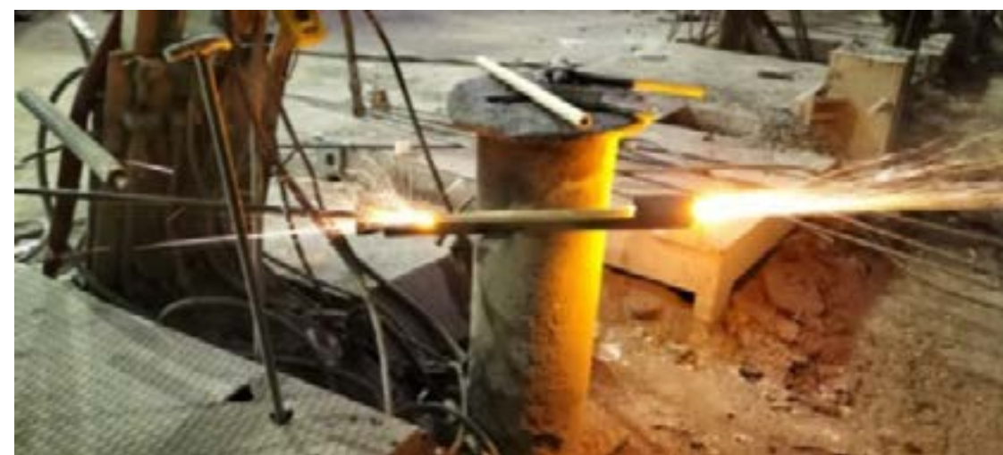
Fig. 5. New method developed for the ignition of the oxygen lances. This procedure avoid the risk of burns and contact with hot substances for the operators
