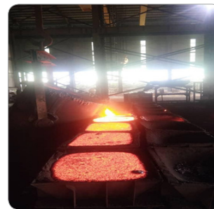
Recovered Alloy Casting Process
