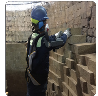
Exoskeleton 2: Picture of the second type of exoskeleton that was developed, for an operator that is mounting bricks in a position higher than the shoulders.
