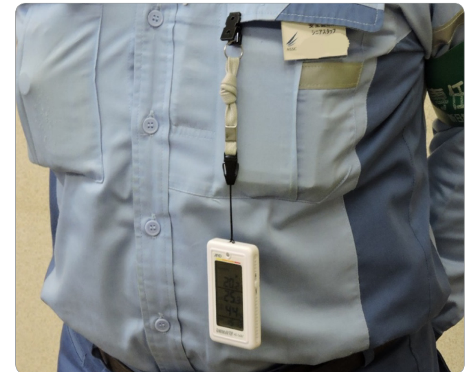
Photo 1: portable WBGT meter
