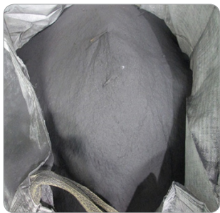
Metal Oxide Dust generated by Acid Regeneration
