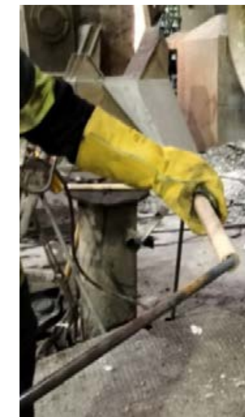
Fig. 2. Method of ignition prior to tool development. Risk of burns and contact with hot substances
