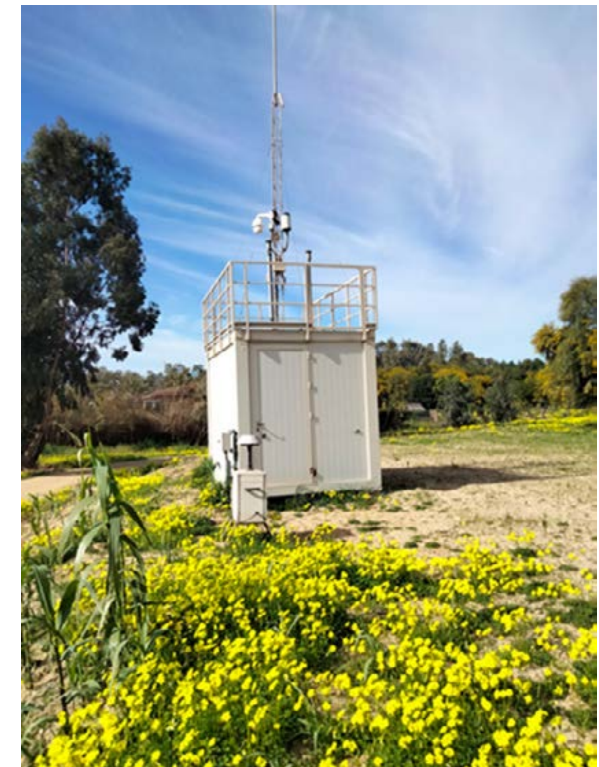
Image 5. Air quality measurement station.
