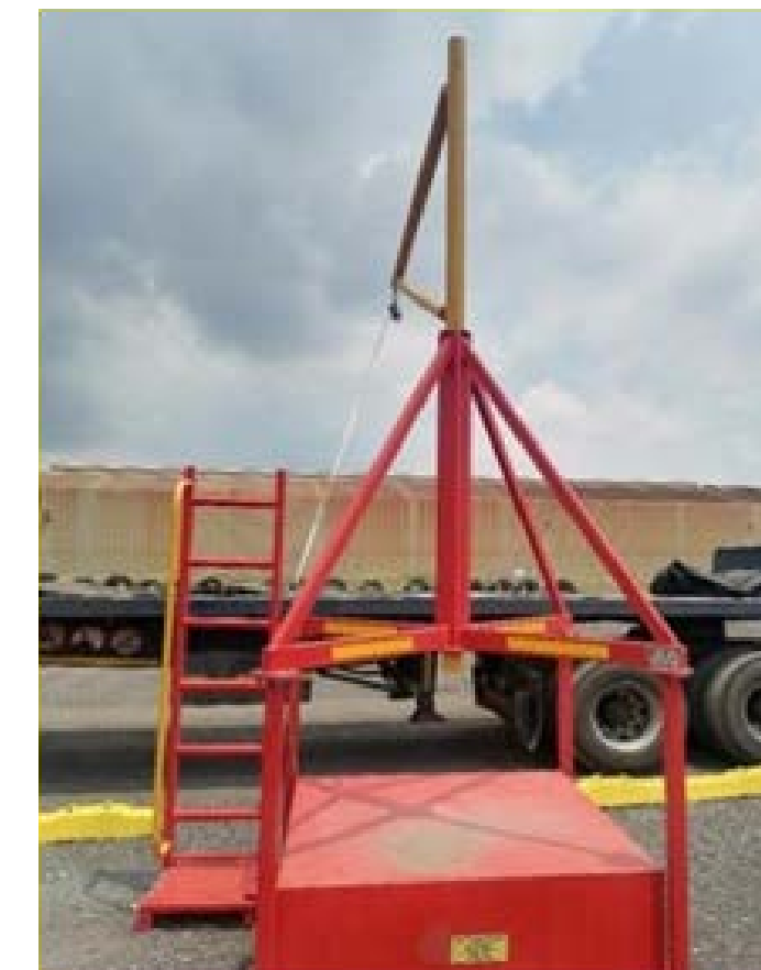
T-Stands fitted with a fixed ladder and retractable lanyard for driver safety
