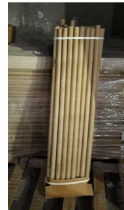
Fig. 1. Cardboard cartridges, which are used for the ignition of the thermal lances
