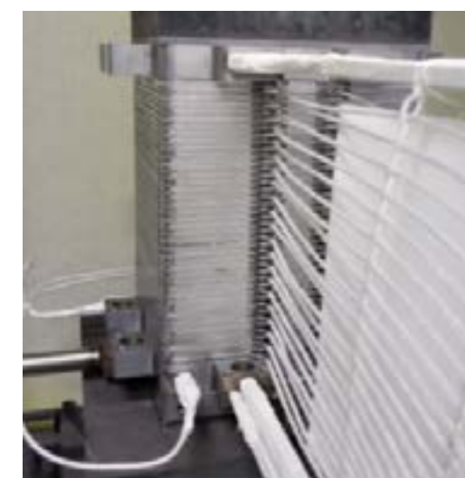
1KW SOFC stack with 460FC separator plates
