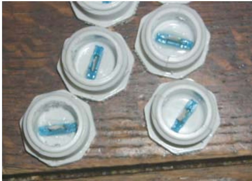
Figure 12. Close-up view of the chloride sensing insert.
