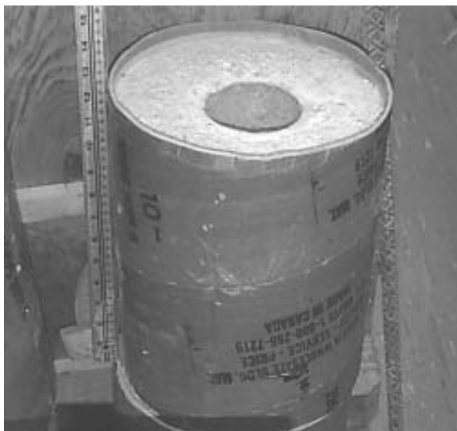
Figure 8. This test cylinder allows ponding of chloride ions in solution. The ions then propagate through the cylinder eventually reaching the fiber optic chloride sensor.
