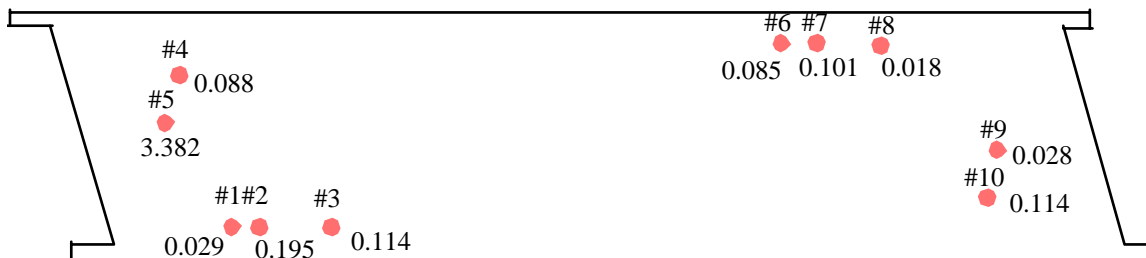
Figure 19.a. Baseline power readings for sensors within bridge A6059.
