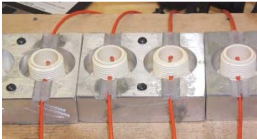
Figure 5. Optical fibers are glued into place and threaded through drilled holes in the PVC screw on cap.
