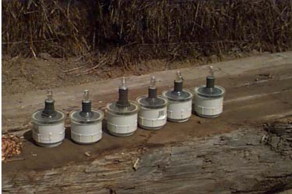
Figure 11. The length of the sensor housing's throat may be modified.
