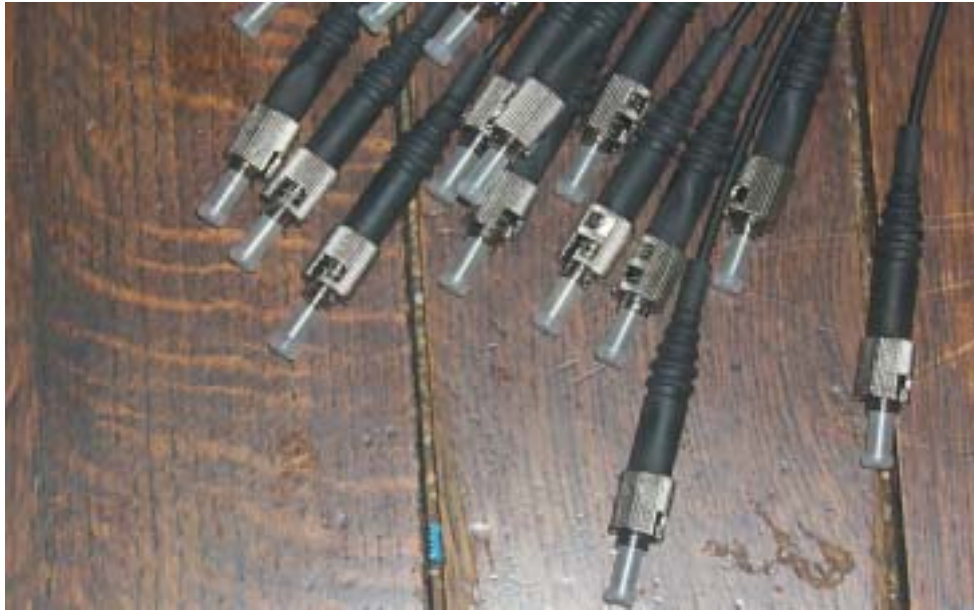
Figure 13. Multimode 960 \mu\text{m} diameter polymer optical fiber with ST connectors is used.
