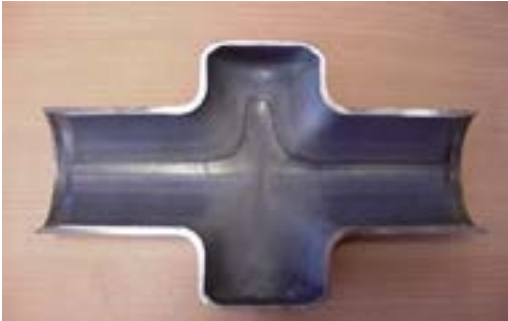
Deformation of the weld (1.4003).
