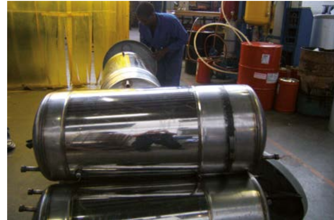
Welded tank, grade 441, S. Africa. Picture courtesy of SunTank, Pretoria, S. Africa
