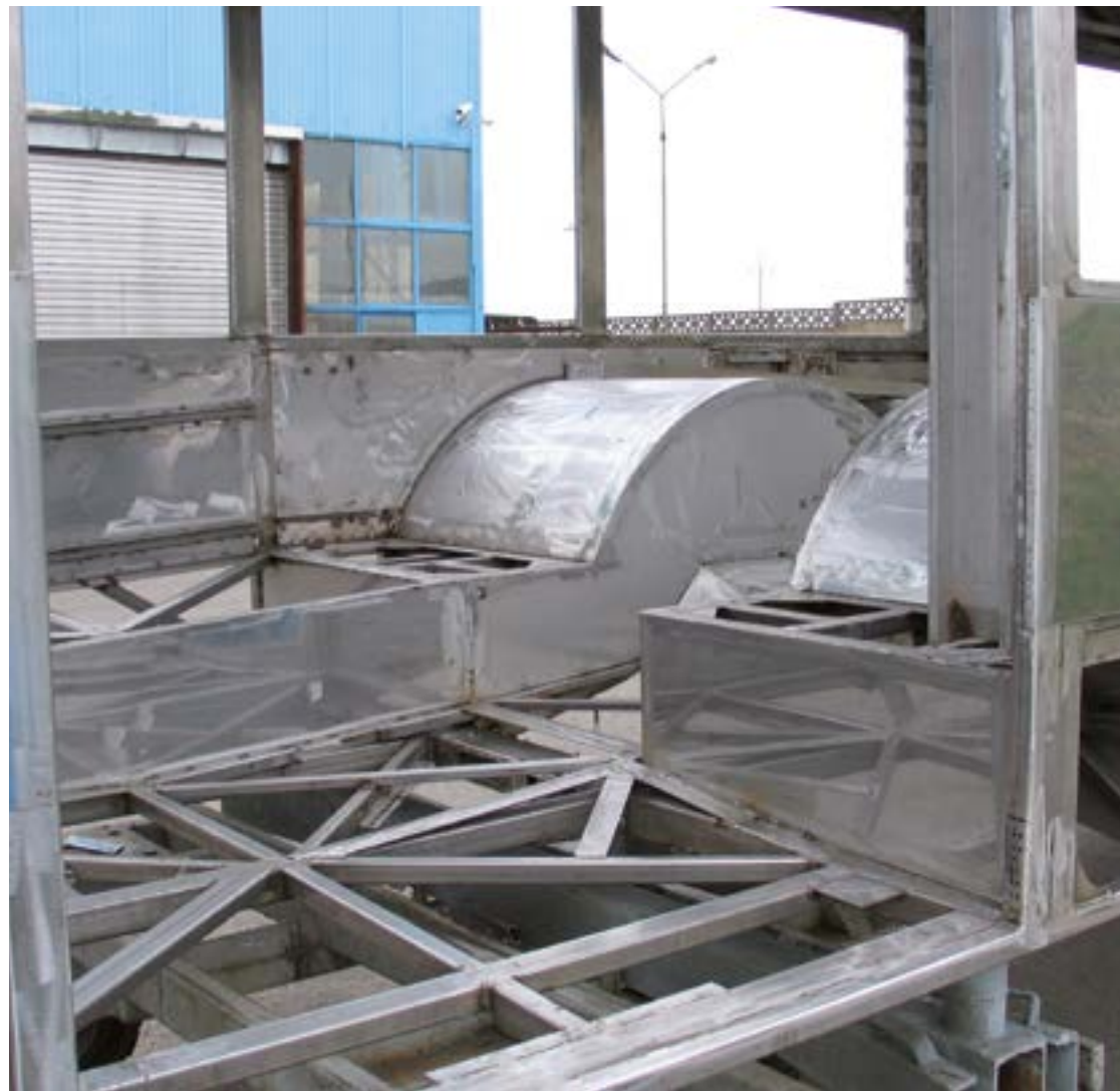
Welded structural frame in grade 1.4003. Picture courtesy of Solaris Bus & Coach Co., Poland
