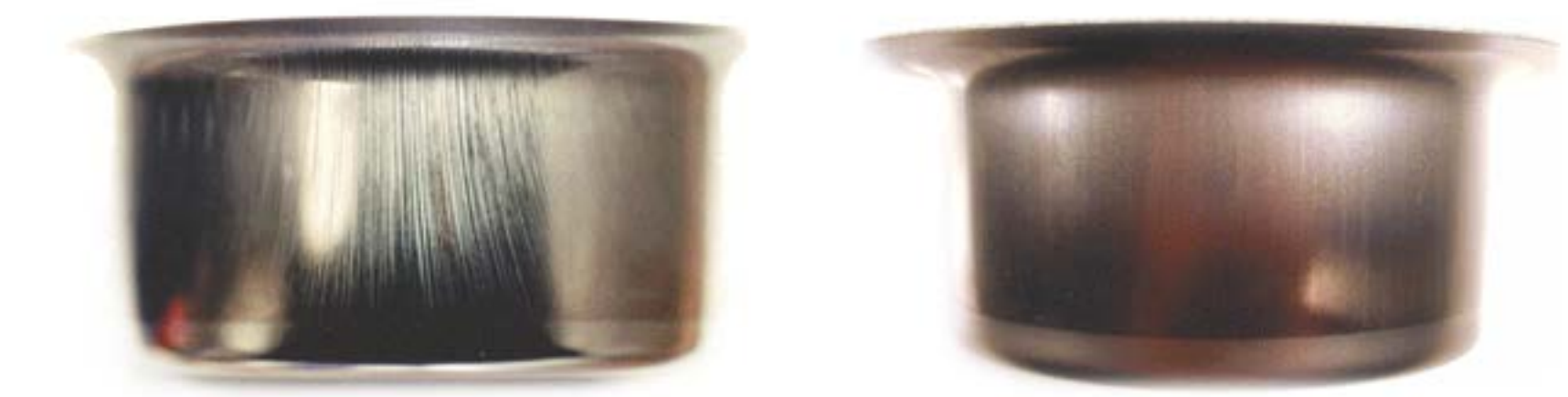
With and without surface defect. Pictures courtesy of Aperam, France
