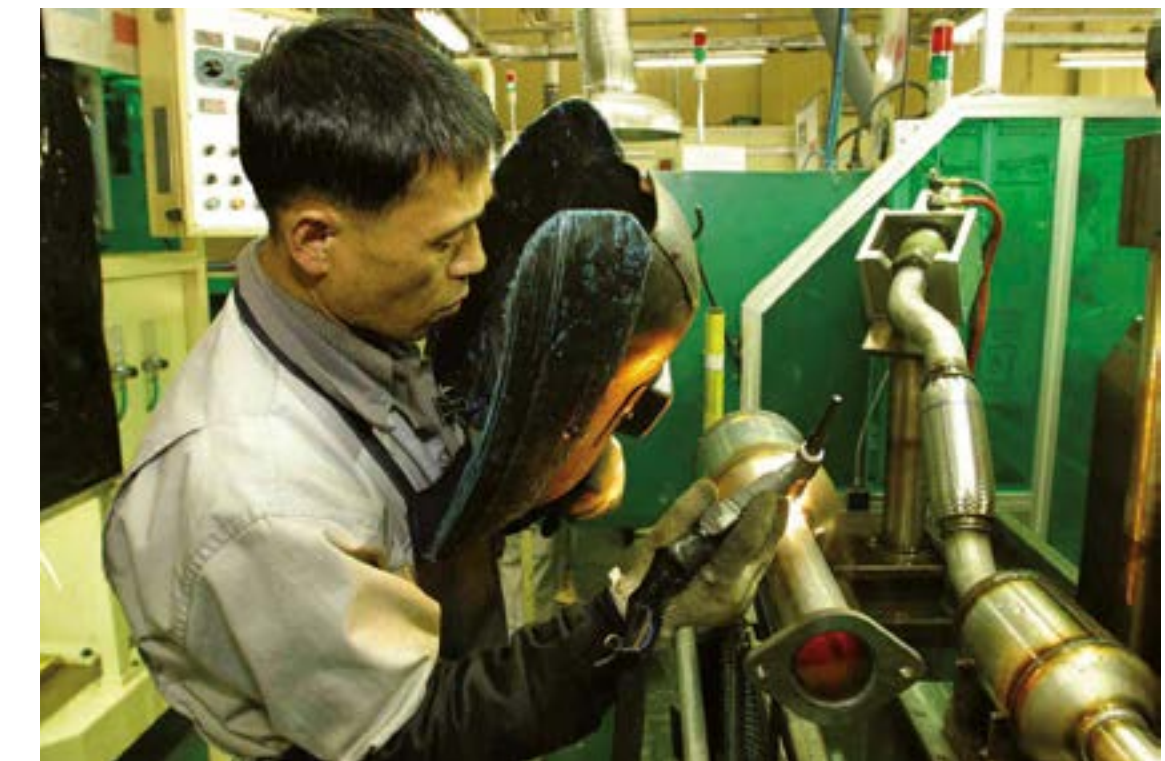
Exhaust system welding, grade 439, S. Korea. Picture courtesy of Faurecia, Nanterre, France
