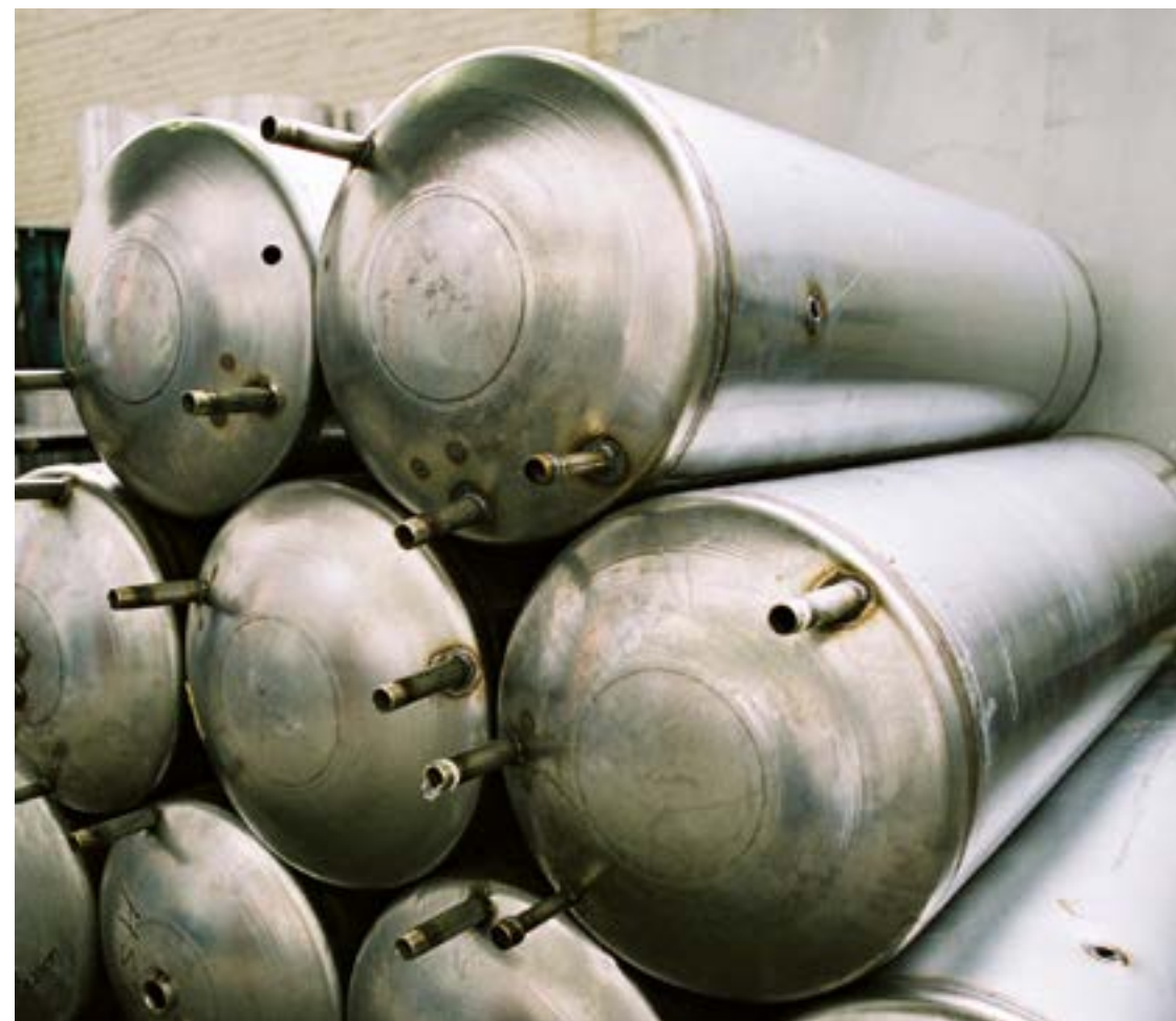
Stamped top and bottom of boilers, in grade 441, S. Africa. Picture courtesy of SunTank, Pretoria, S. Africa
