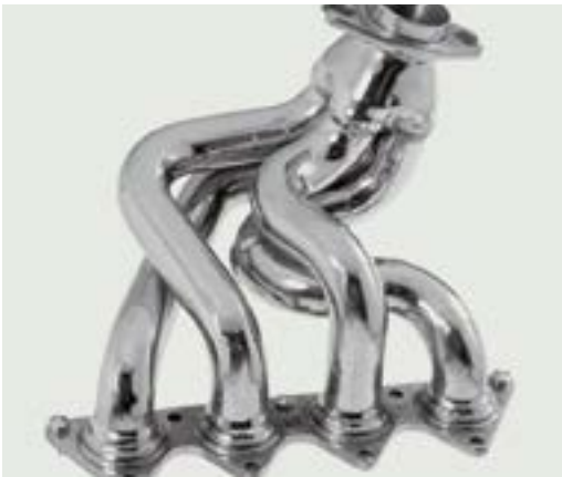
Welded bended tubes of a manifold, in grade 441. Picture courtesy of Faurecia, Nanterre, France;
